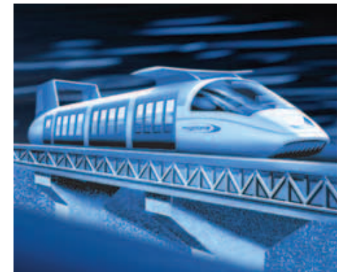
Figure 4.11: With a maglev train, there is no contact between the moving train and the rail—and thus there is little friction.
