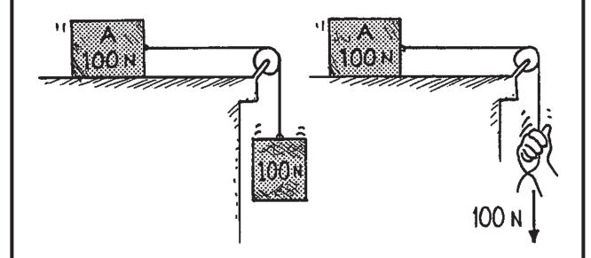
IN BOTH CASES AN APPLIED FORCE OF 100 N ACCELERATES THE 100-N BLOCK.
